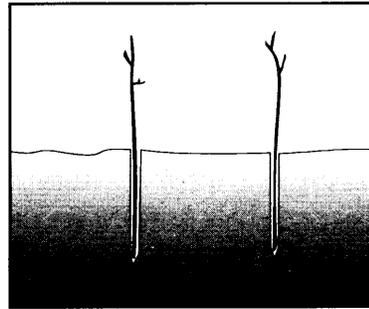
2. Insert willow cutting to the bottom of the hole.
