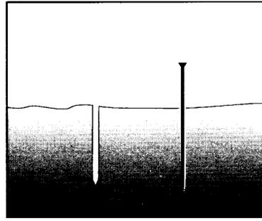
1. If soil is too hard for direct cutting placement, use a planting bar to create a hole. Make hole half the length of the cutting.
