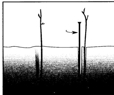
3. Re-insert the planting bar adjacent to first hole and move bar toward willow cutting to close hole.
